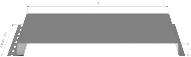
METAL BLOCK- 12 in (305 mm) x 1 in (25.4 mm) x custom length up to 60 ft (18.29 m)
