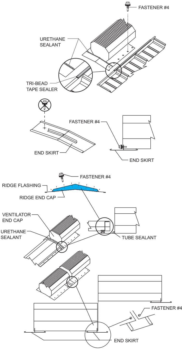
After Tri-Bead tape sealer has been applied to top of outside closures, install ventilator in proper location. Be sure to center in opening. Attach ventilator to outside closures with Fastener #4 on 6" centers. Use tube sealant to seal between the outside of the ventilator and the end skirt.
