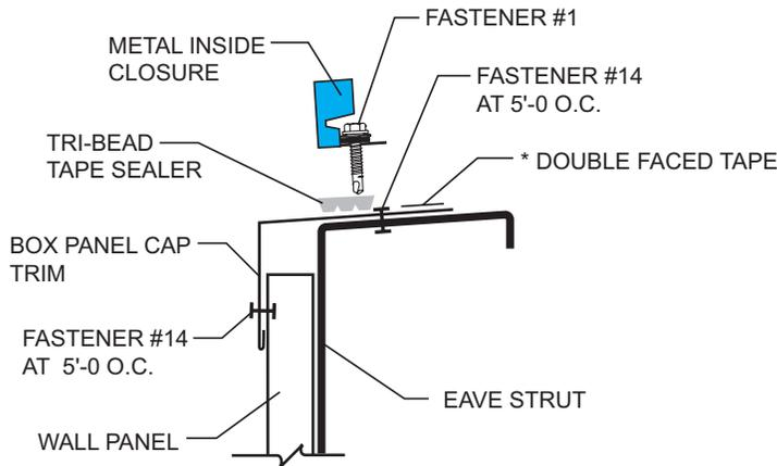
Using Fastener #1, attach the first inside closure to the eave strut, locating the face of the inside closure with the steel line. **NOTE THAT THE FIRST INSIDE CLOSURE MUST BE FIELD CUT IN HALF TO FILL THE VOID UNDER THE PARTIAL RIB.**
