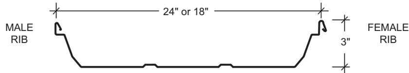
Coverage Width - 24" with minor ribs - prepunched 6 holes
