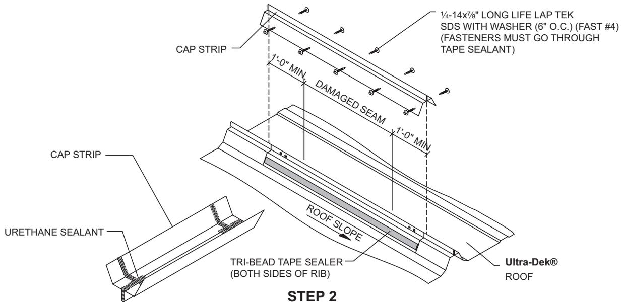
1. Install a continuous run of Tri-Bead tape sealer to both sides of damaged panel rib.
