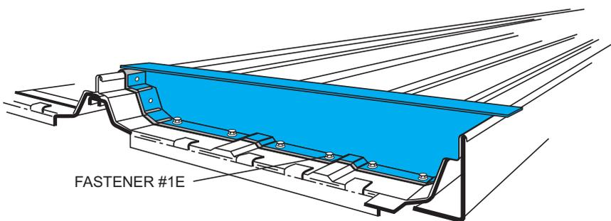
Push the other end of the outside closure into position and align the holes with the awl. Remove the awl and install Fastener #1E in all remaining holes except for the hole at the panel seam. **Do not install the panel seam fastener at this time.**
