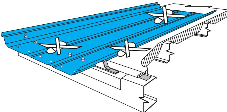
**NOTE: IT IS ESSENTIAL THAT THE ERECTOR MAINTAIN A 24" MODULE AT THE EAVE, WITH THE PROPER INSTALLATION OF THE INSIDE CLOSURES AND BY INSTALLING FASTENERS IN THE PROPER SEQUENCE.**
