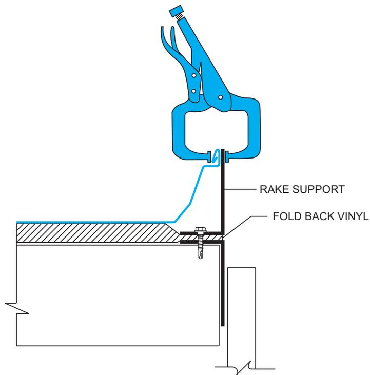
After laying the last insulation run, install the rake support over the insulation along the steel line. Lay the last panel run. Temporarily attach the male leg to the rake support with vise grips.
