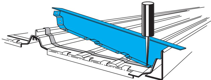
Install back-up plate and panel clips. Go to the previously installed ridge panel and peel protective paper from tape sealer. Apply tape sealer to the ridge panel just installed. Be sure to seal to the mastic on the previous panel.
