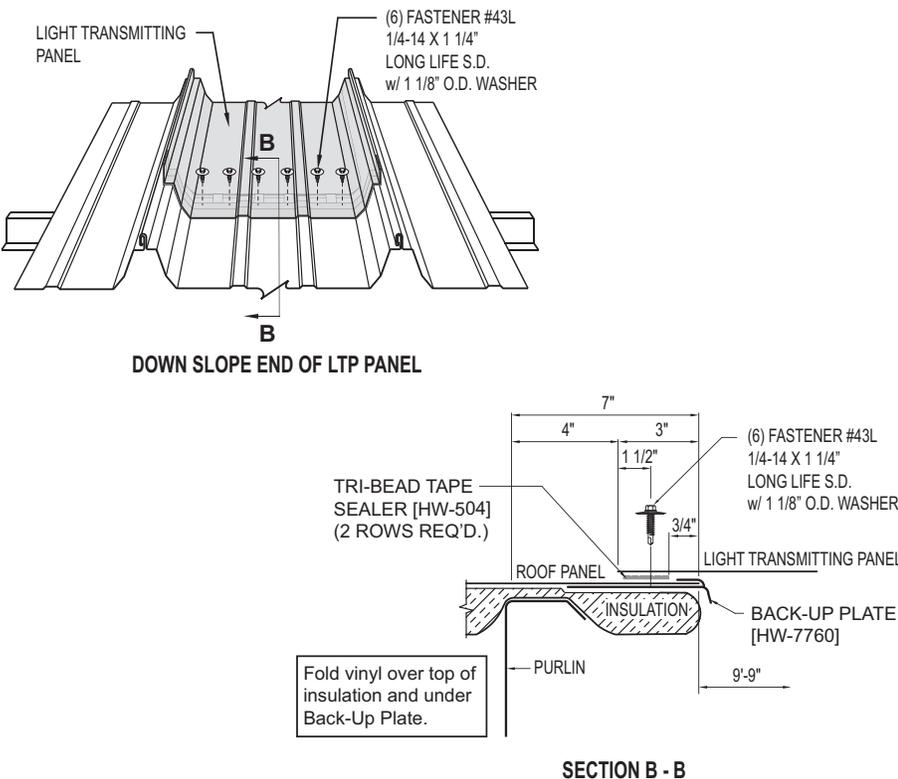
At the down slope end of the LTP, install six #43L fasteners through the LTP, the metal panel and into the back-up plate. Fasteners should be 1 1/2" up slope from the edge of the LTP and spaced evenly across the flat of the panel as shown in the bottom two drawings.
