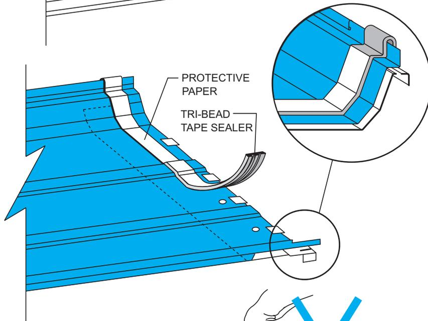
Place Tri-Bead tape sealer over the entire width of the panel. It must be centered directly over the pre-punched holes, following the panel configuration.
