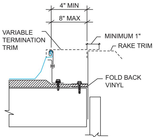
If the panel ends 2"- 4" away from the rake support due to an out-of-square condition or other factors, simply install the panel clips. This system allows for the roof to be trimmed in the high.
