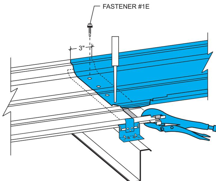
Position female lip of upper panel over rake support, while holding male side of panel up away from the tape sealer. Using an awl, align the hole nearest the female side of the top panel with the corresponding hole in the lower panel and the back-up plate.
