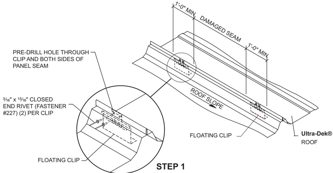
1. Repair cap must extend 1'-0" above and below the damaged area.
