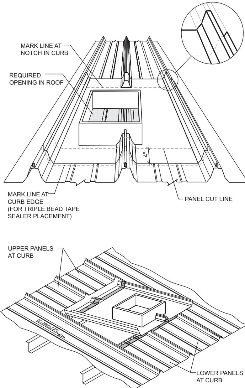
Once curb is ready to be installed, lay curb on roof and align opening in the curb with the exact location the opening is required in the roof. At the up slope end of the roof curb, the roof panels will be cut on a line even with the beginning of the notch at the vertical leg on each side of the roof curb. Secondly, trace a line along the down slope edge of the roof curb. The roof panels will be cut on a line 4" up slope from this line.
