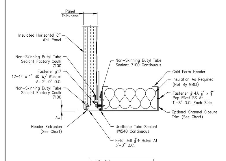
The interior leg of the Installed Channel Closure Trim is to be oriented  $\left(\pm\frac{1}{8}"\right)$  to match the interior leg of the Header or Jamb.
