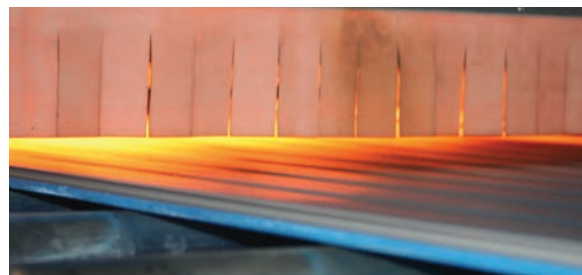
The steel moves through the pre-heat oven so that the foam aggressively adheres to the metal.
